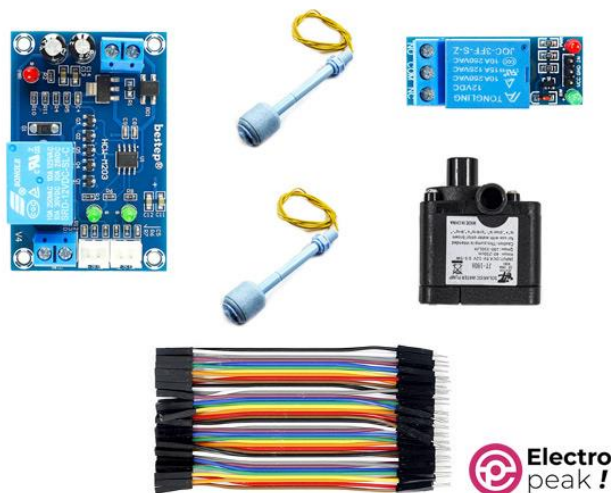
Automatic Water Level Controller Module-Required-Materials
