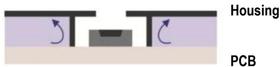
**Figure 12.** The sensor is isolated from the air inside the housing, which minimizes the impact of the air inside the housing on the sensor.
