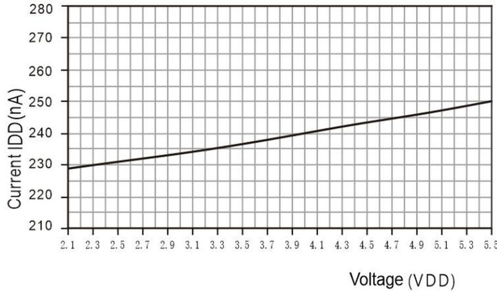
**Figure 7** The relationship between typical supply current and supply voltage at 25°C Curve (sleep mode), please note that the deviation of these data from the displayed value may reach ±50% of the displayed value. At 60°C, the coefficient is about 15 (Compared with table 2)
