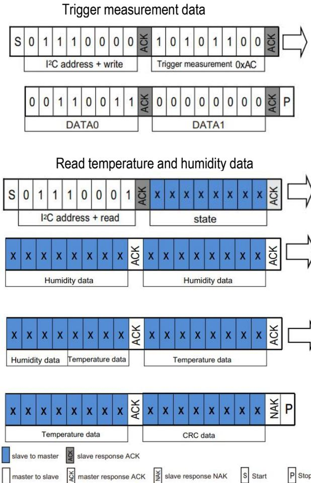
Note: The sensor needs time to collect. After the host sends a measurement command (0xAC), delay more than 80 milliseconds before reading the converted data and judging whether the returned status bit is normal. If the status bit [Bit7] is 0, it means that the data can be read normally. When it is 1, the sensor is busy, and the host needs to wait for the data processing to complete.
