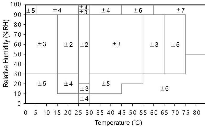
Figure 5. The typical error of humidity in the range of 0~80°C, unit: (%RH)
