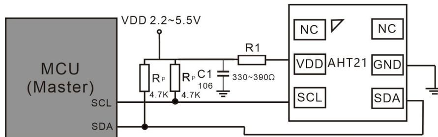
**Figure 16.** Typical application circuit
